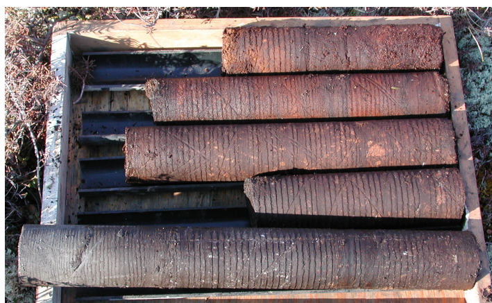
Figure 2. Frozen soil core samples from the Norman Wells site. The right end of the upper core is the surface and the left end of the lower core is the mineral layer below the basal peat.
